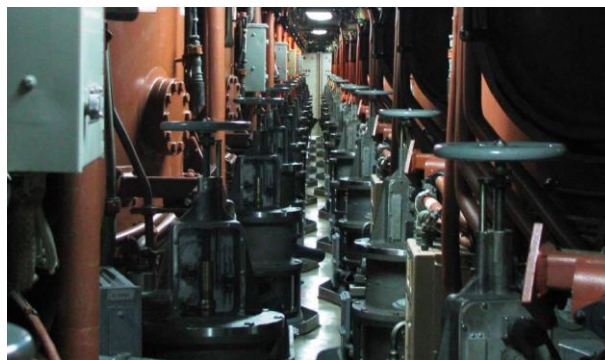
The missile compartment of an Ohio-class nuclear submarine. The entrances to the crews' sleeping quarters are to the left and right, reached by walking between two missile tubes.
